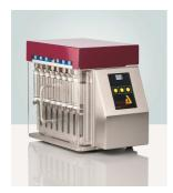
The PT-SP multi-syringe pump is designed specifically for parallel sample withdrawal and dosage of media from a dissolution bath into open vials inside a fraction collector. It is equipped with up to 8 replaceable 10ml high precision glass syringes. Each syringe is connected to a 3-way pinch valve for media flow control. The drive of the syringes is carried out simultaneously by a stepper motor. All syringes are rigidly connected to the common sturdy drive bar
