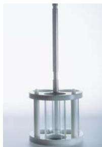
"B" Basket, (Test "B" EP <2.9.1.2> and USP <2040>) 33 mm diam., used to test bigger samples order no. 105-2014 incl. glass tubes and disks
