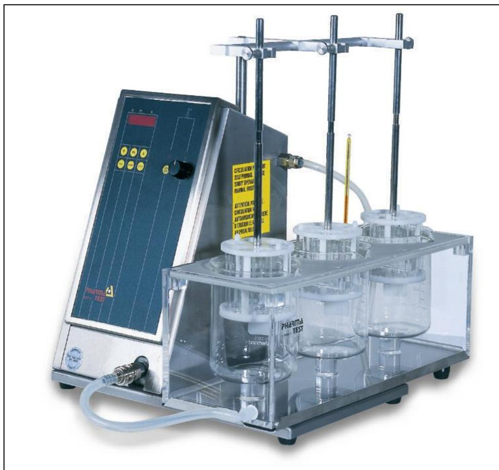
The **DIST 3** is essentially a three station version of the PTZ S Disintegration Test Apparatus. This instrument offers the attractive combination of cost efficiency and high sample throughput. All three standard disintegration baskets are suspended from a common drive arm which is attached to a single drive motor. All three baskets are in operation at any one time. The orientation of the baskets, which are all USP<701/2040>, EP<2.9.1/2.9.1.2>, JP and others compliant, is from front to back.
