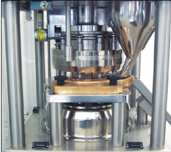
Automated Version with Force Sensing Attachments
