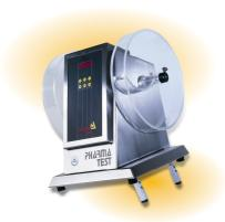
PHARMA TEST AG Siemensstrasse 5 D-63512 Hainburg (GER) performed following the individual monographs of the Pharmacopoeia. When finished the samples have to be de-dusted an weighted again. Actually the difference between the weight before and after the test is determined as Friability which usually should not exceed 1%. Tablets of a diameter more than 13 mm are tested while the apparatus is lifted at one side for about 10°.
