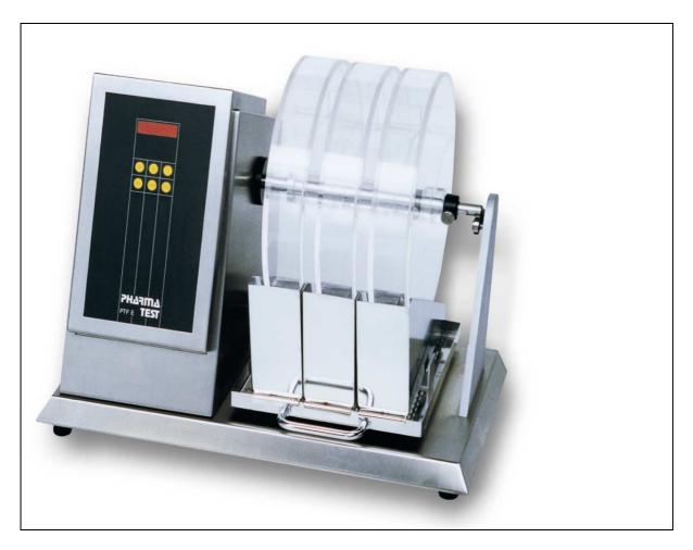
The **PTF 30ERA** is a multiple drum Friabilator with automated sample discharging option at the end of a test run. It is equipped as standard with 3 Perspex (plexi glass) Friabilator drums attached to a single drive axis. A DC motor is used to rotate the drums, the rotation speed can be selected as well as the number of drum revolution or the total testing time.
