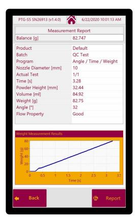
The test results are displayed on screen and can be recalled at any time from the integrated result database. The results are expressed numerically and graphically. Furthermore the flow behaviour is evaluated according to the USP/EP criteria.
