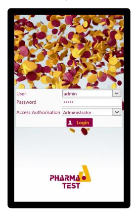
Log on to the instrument by selecting your user from the list and by entering your password. You can either use the on screen keyboard or you can connect any standard USB keyboard to the instrument to enter your data. Depending on your access level, you can log on with different authorization levels. This access authorisation level determines which menus displayed and which settings can be changed.
