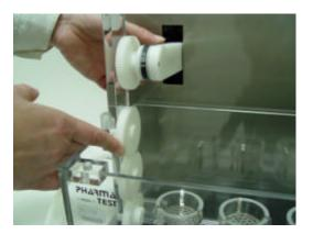
Adjust the supports inside the bath previous to test start
