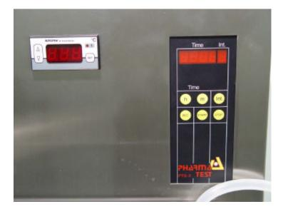
The keyboard includes the timer display, the time setting keys and start/stop key.
