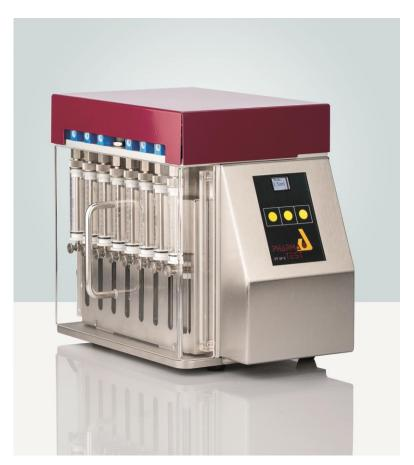
The PT-SP multi-syringe pump is designed specifically for parallel sample withdrawal and dosage of media from a dissolution bath into open vials inside a fraction collector. It is equipped with up to 8 replaceable 10ml high precision glass syringes. Each syringe is connected to a 3-way pinch valve for media flow control. The drive of the syringes is carried out simultaneously by a stepper motor. All
