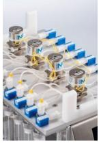
syringes are rigidly connected to the common sturdy drive bar.
