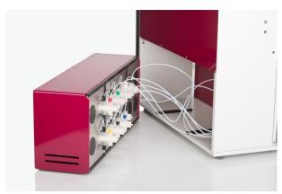
Unlike most systems the DSR-M does not use syringes but valve-less piston pumps. These pumps do not need any time consuming prefilling and emptying cycles and change of valve positions. Also the dead volume is much smaller compared to conventional syringes and valve installations.
