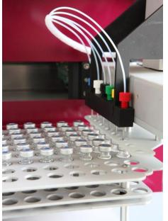
To offer the highest volume precision, between six and thirteen piston pumps are used for sample removal and media refilling (optional), one dedicated pump for each channel. No time consuming pump calibration is needed. The advanced design of the system means that it is always ready for operation. The pumps are integrated into the DSR-M as a compact CAT-M pump module.
