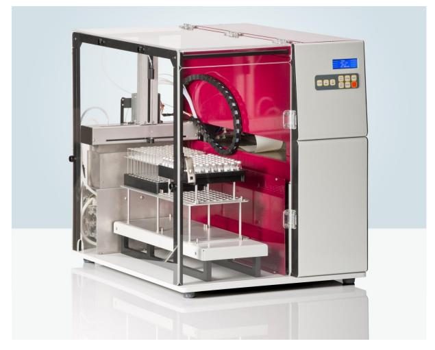
The DSR-M dissolution sampling robot is designed specifically for the sample transfer and sample processing from a six to twelve vessel dissolution bath. This unique versatile instrument allows samples to be collected over very short time intervals. The DSR-M can be equipped to collect, dilute or process samples for following UV-Visible or HPLC measurements. It can also be used for dissolution
